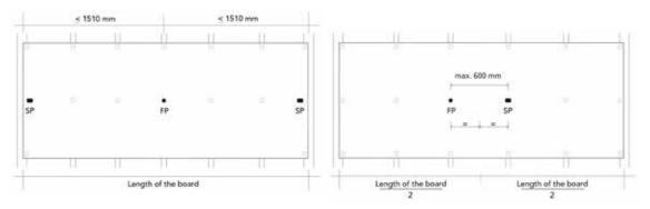
Figure 5: Combination of fixed and slotted point in asymmetric way
