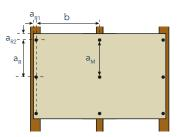
Maximum fixing distance (mm) screws a for different c.t.c. distances (b) of the vertical sub-construction ( $k_{mod}$ : 0.90 / 1.00 / 1.10)
