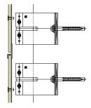
Aluminium sub-construction with closed horizontal joint
