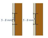
Timber sub-construction with closed (left) and semi-closed (right) horizontal joint
