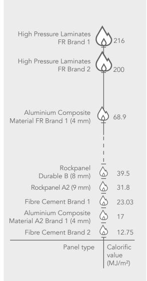
With a low calorific value, Rockpanel A2 board material sets the benchmark for very low combustion heat.
