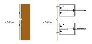
Timber sub-construction, open horizontal joint
