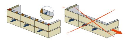
To be able to calculate the fixing distances as with open joints (which means reducing the wind load with pressure equalisation and achieving wider fixing distances), application needs to be done according the following pre-conditions:
