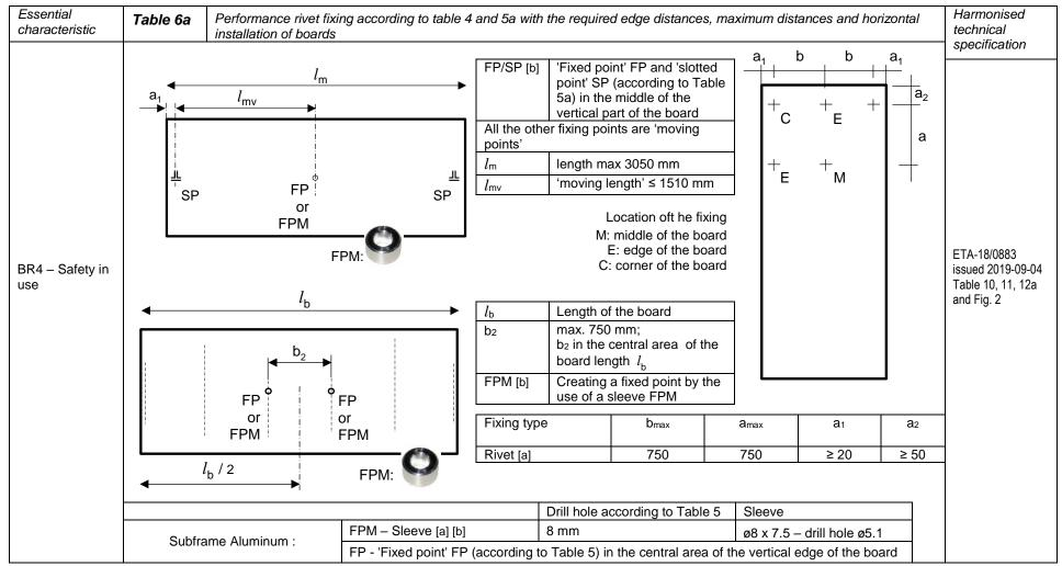
[a]: For correct fixing (FP and FPM) a riveting tool with rivet spacer must be used (e.g. 0.3 mm).
