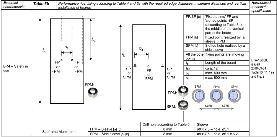
[a]: For correct fixing (FP, FPM, SP and SPM) a riveting tool with rivet spacer must be used (e.g. 0.3 mm). [b]: Subframe aluminium
